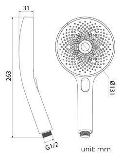
Flow Rate: 2.0 GPM / 7.6 LPM
